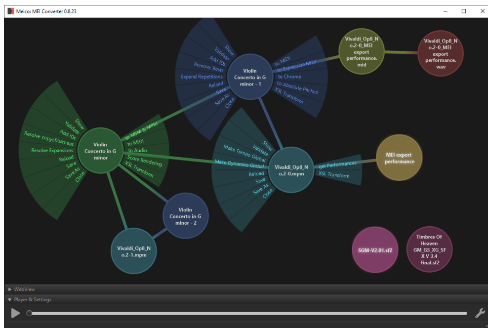
Figure 1. Screenshot of the meicoApp. From the MEI data (left, green) MSM (dark blue) and MPM (light blue) are exported. The MPM here contains one performance, “MEI export performance”, from which the MSM can be rendered “to Expressive MIDI” (top, yellow). The MIDI data is rendered to audio (top right, red). At the bottom right, two external soundfonts are included, the left one is activated.
