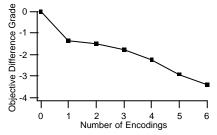
Figure 1. Effect of multiple encodings on audio quality. The Objective Difference Grade measures perceived difference in quality between a reference and test signal.
