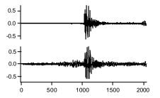
Figure 2. Original signal(top) and pre-echoes(bottom) from castanets with block processing of 2048 samples.
