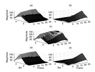
**Figure 5**. LS estimation of overlapped harmonics. (a) The magnitude spectrum of a harmonic of the first source in the overlapping T-F region. (b) The magnitude spectrum of a harmonic of the second source in the same T-F region. (c) The magnitude spectrum of the mixture at the same T-F region. (d) The estimated magnitude spectrum of the harmonic from the first source. (e) The estimated magnitude spectrum of the harmonic from the second source.
