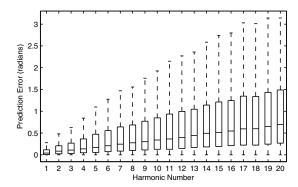
**Figure 4**. Box plots of phase change prediction error as a function of harmonic number. Results are calculated using 40 five second instrument performances, with error (in radians) calculated as absolute difference between true change in phase from frame m to m+1 and predicted change in phase for frame m.
