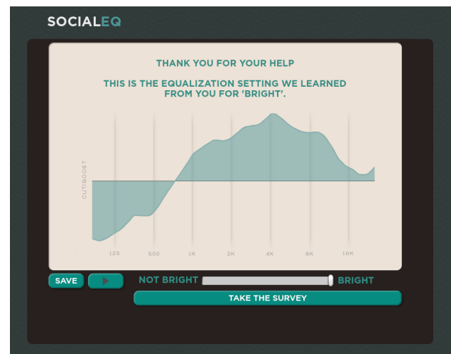
Figure 2. The equalization curve and control slider learned for "bright" in a single session.
