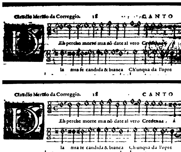
Figure 7. The binarization results with B1 (above) and B2 (below). The B2 option was clearly more appropriate for removing the bleed-through, in particular where the ornate letter is printed on the other side.
