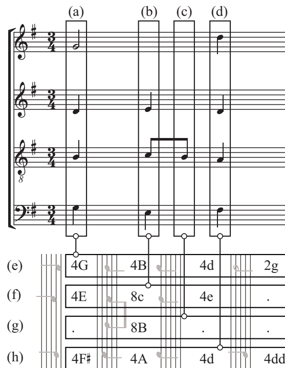
Figure 1. An ENP score displayed as graphical music notation (top) partitioned into harmonic slices (a–d) which are converted into kern records (e–h).
