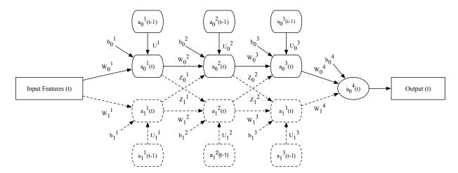
Figure 2: Overview of the proposed bi-directional recurrent neural network (BDRNN) and recurrent neural network (RNN). Solid lines represent the RNN connections and dashed lines are additional BDRNN connections. Tan sigmoid layers are shown as curved rectangles and soft max layers are represented by circles. The weight matrices are denoted as W, U and Z and the biases as b. The output of layer two of the backwards directional recurrent neural network is denoted by  $a_1^2$ .
