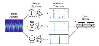
**Figure 1**: Overview of proposed method. Features are input to individual neural networks for each instrument, resulting in activation functions. Drum onsets are found by peak-picking the activation functions.
