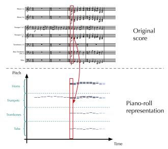
**Figure 3**. *Piano-roll* representation of orchestral scores. The *piano-roll* pr is a matrix. A pitch p at time t played with an intensity i is represented by pr(p,t)=i, where 0 is a note off. This definition is extended to an orchestra by simply concatenating the *piano-rolls* of every instrument along the pitch dimension.
