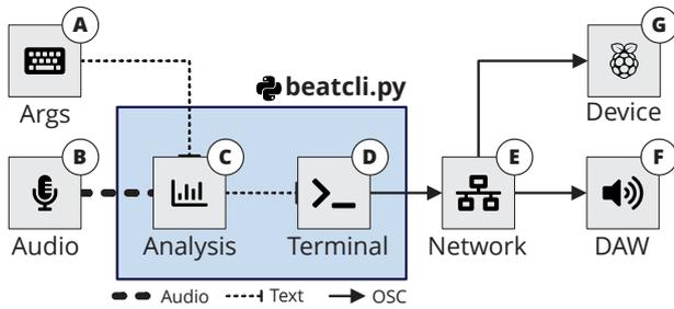
**Figure 2.** A block diagram of the *beatcli.py* terminal application. (A) Input arguments. (B) Audio input. (C) Audio analysis. (D) Terminal output. (E) Network output. (F) Receiving software. (G) Receiving hardware.
