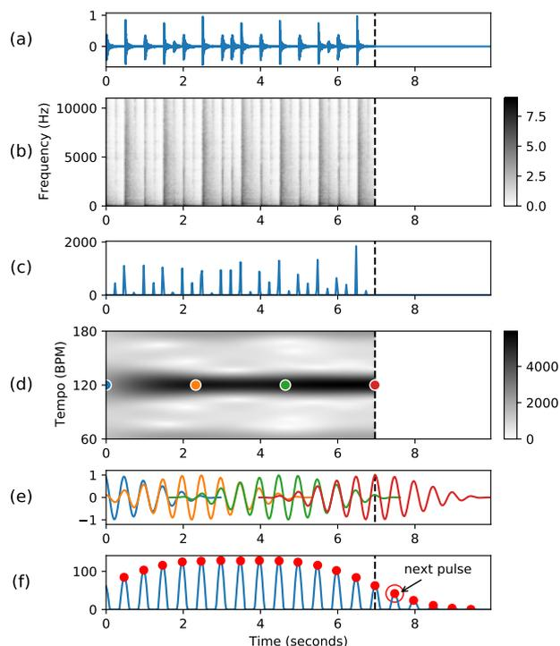
**Figure 1.** Illustration of the PLP computation pipeline and its real-time implementation. (a) Waveform. (b) Spectrogram. (c) Novelty. (d) Tempogram. (e) Kernels. (f) PLP.
