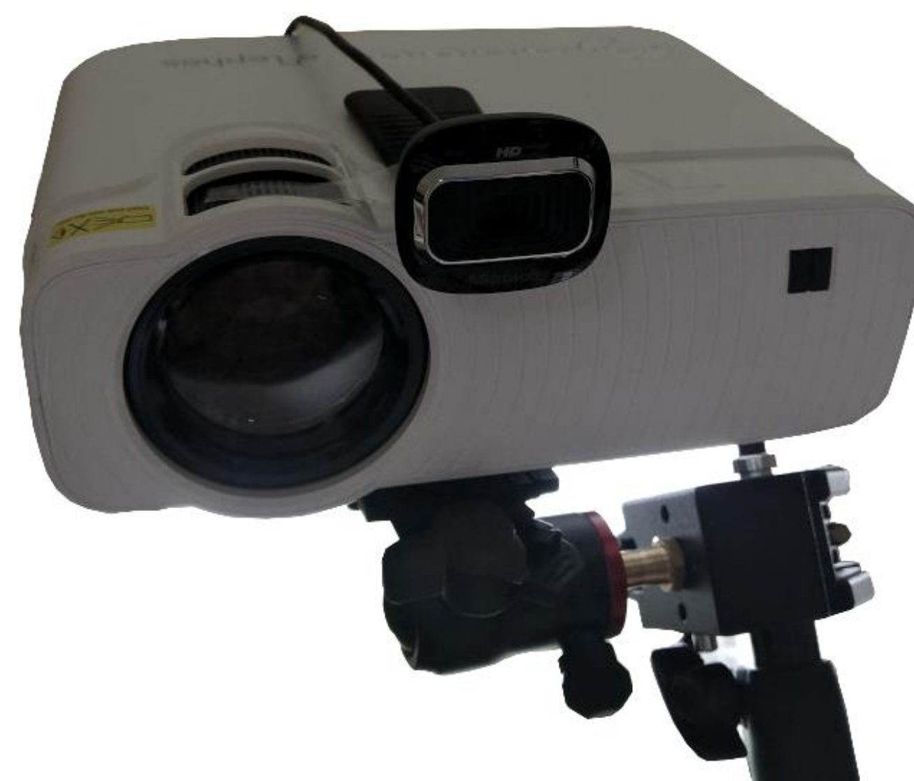
Left: Hardware setup with projector and webcam (for calibration) on a tripod. Right: Visualizations using 1) color, 2) a tachometer needle, and 3) pie charts.
