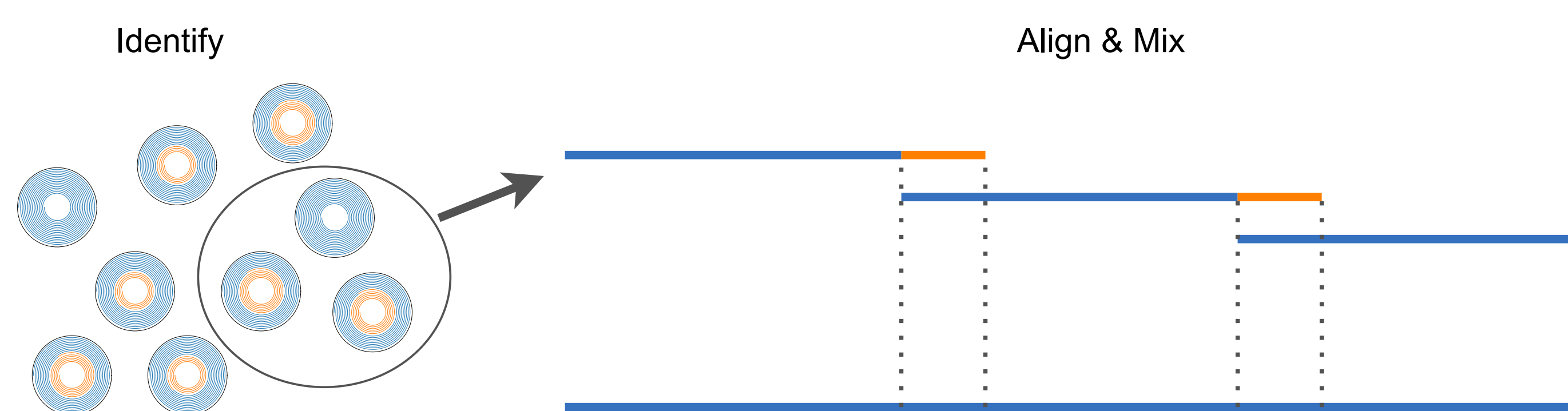
Fig: Overlapping discs need to be identified from a large set of disks. The overlapping parts (in orange) need to be precisely aligned. A mixing step reassembles the original recorded event. Identification, alignment and mixing is problematic due to speed differences and speed variabilities in overlapping discs.
